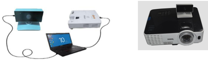
Hardware installation Notice: Please reference the suggested distance table below. It is recommended that the signal receiver be placed on the projector.
